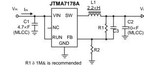
R2  $\delta$  200K& is recommended Place C1 closed VIN/GND. Without via hole is recommended.
