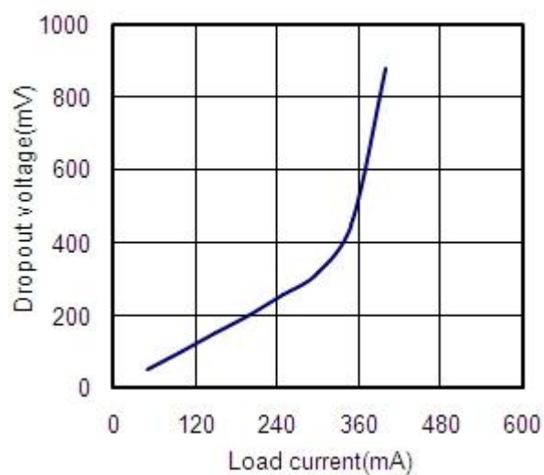
Load Voltage vs. Dropout voltage
