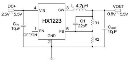
\* The output voltage is adjustable: Vout= 0.8V · [1 + (R1/R2)]
