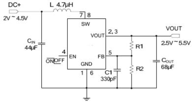
\* The output voltage is adjustable and set by R1 and R2: Vout =  $1.2V \cdot [1 + (R1/R2)]$ .
